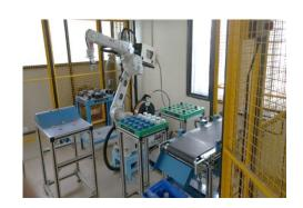
ABB 1520 ID 6-DoF Industrial Robot with Welding Fixture, Matrix table & Conveyer
