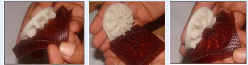
Molding and casting of polyurethane parts
