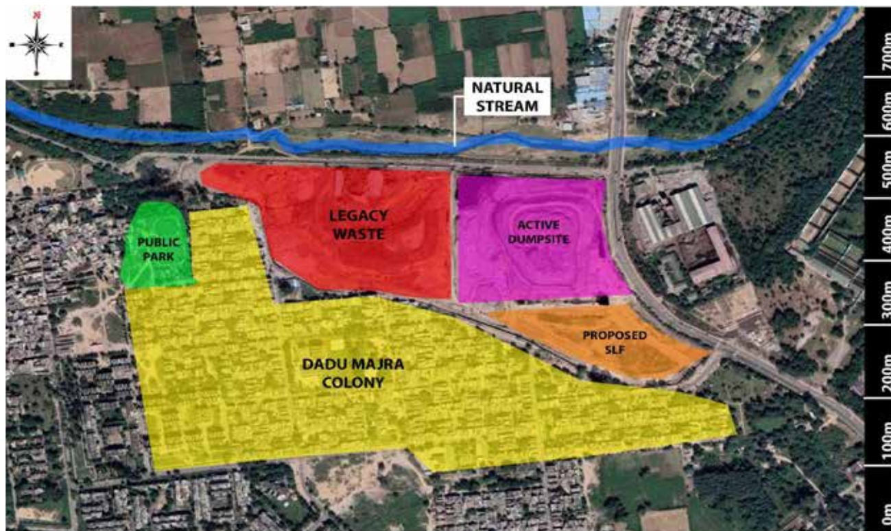
Figure 3 - Showing the surroundings and parts of Dadu Majra Dumping Ground (Source - Google Earth and Author)
